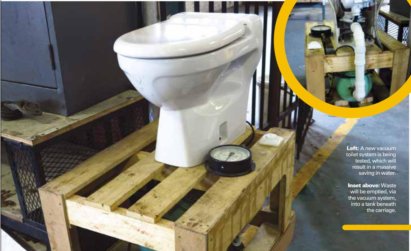
**Left:** A new vacuum toilet system is being tested, which will result in a massive saving in water.
