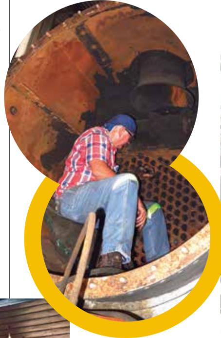
**Above:** Descaling the locomotives' boiler tubes is a significant task.
